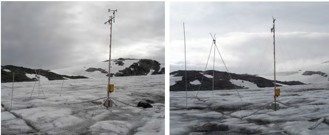
Figure 6-6 The AWS site on Midtdalsbreen after the maintenance on 29 th August 2008 (left) and upon arrival on 24 th August 2009 (right). The ice surface sank 3.4 m during this period. Photo: Rianne H. Giesen.
