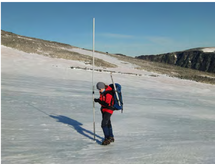
Figure 9-3 Ablation measurements on stake 5 on 15 th September 2009. Photo: Gabrielle Bippus.
