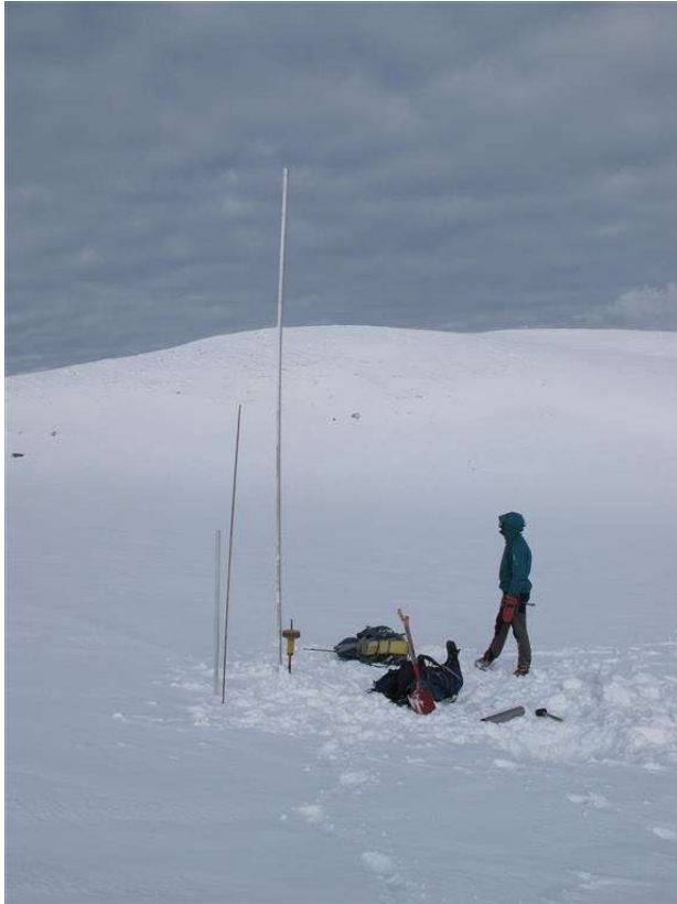
Figure 10-5 Stake position measurements at stake location 7 (two stakes) in September 2015. The surface was covered with fresh snow. See also Figure 10-2. Photo: Liss M. Andreassen.
