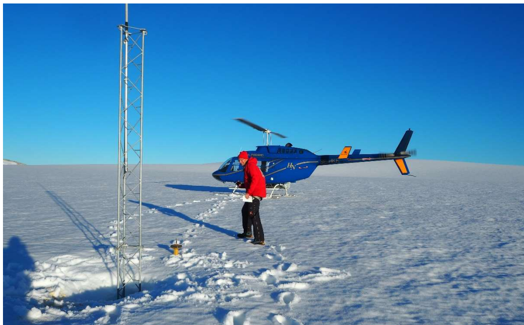
Figure 1-1 Tower used for summer and annual balance on Engabreen in August 2017. Photo: Jostein Aasen.
