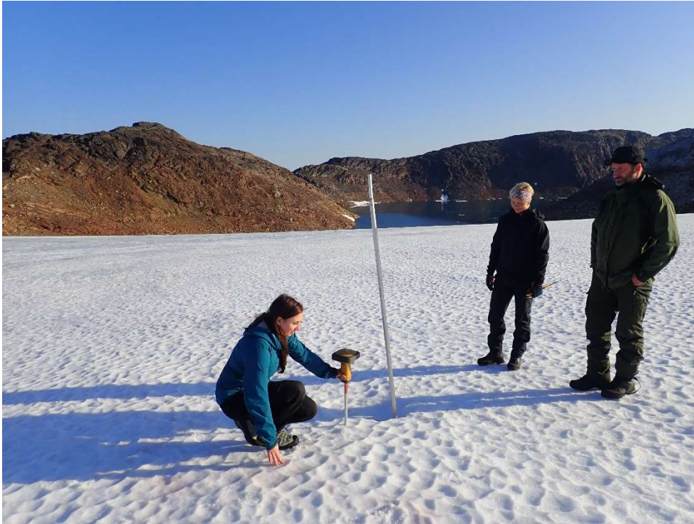
Figure 12-3 Ablation measurements in September 2017 included stake readings and stake positioning by GNSS. Photo: Miriam Jackson.
