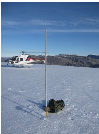
Figure 2-5 Stake reading and GNSS positioning of stake 90 during the ablation measurements on 19 th October. Photo: Bjarne Kjølmoen.
