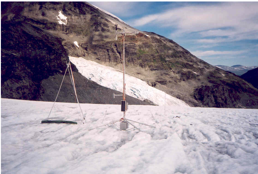
Figure 7-5 The automatic weather station (AWS) at Storbreen, July 2003. Photo: Liss M. Andreassen.
