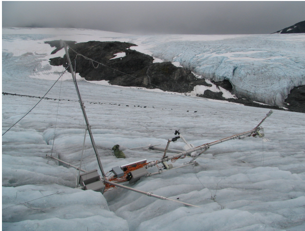
Figure 7-5 The AWS fell down on July 22 nd due to opening of a crevasse. The station was fixed in August. Photo Liss M. Andreassen
