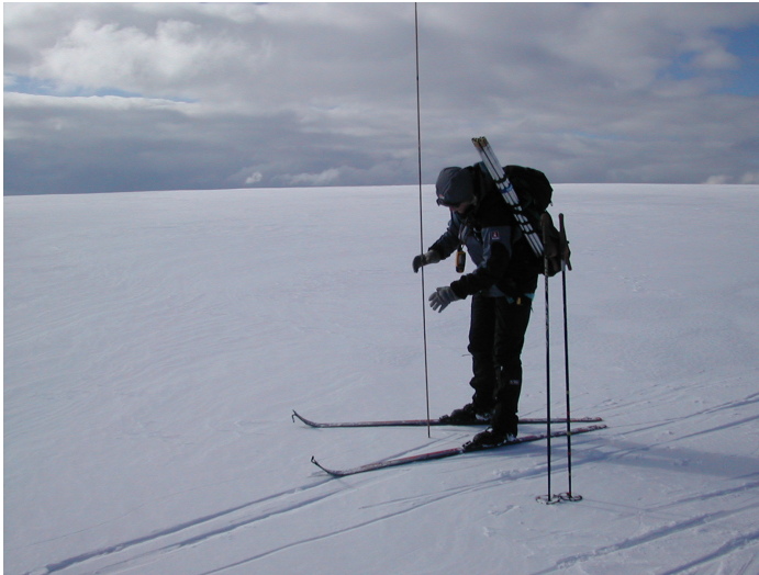
Figure 12-2 72 snow depth soundings were performed in May 2005. Photo: Ole Magnus Tønnsberg.
