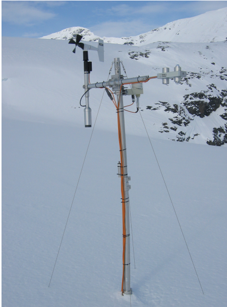
Figure 7-5 The upper arm of the AWS in March 2005. The lower arm was already covered by snow on 2nd January. Photo: NVE.
