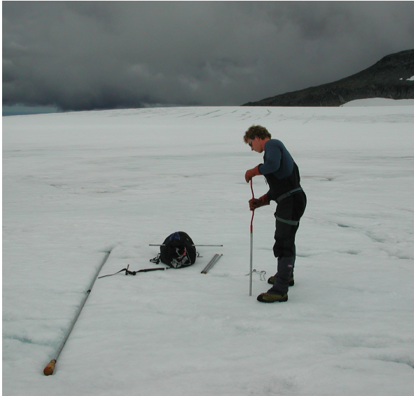
Figure 1-2 Ablation stakes are usually re-drilled during the summer season. Photo: Hallgeir Elvehøy, NVE.
