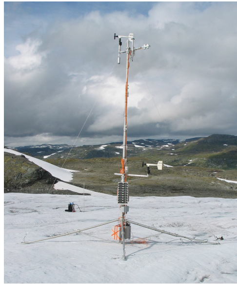
Figure 6-4 The AWS on Midtdalsbreen, 26 th August 2005. Photo: C.H. Tijn-Reijmer.
