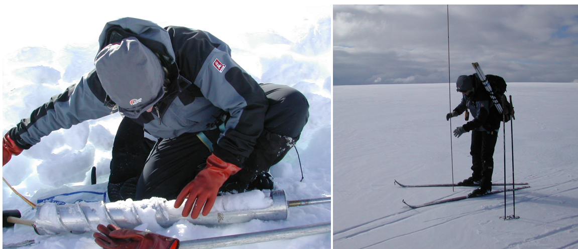
Figure 1-1 Snow depth is normally measured by probing to the previous year's summer surface (right). If the summer surface is difficult to distinguish, particularly in snow-rich winters, snow coring is also used to determine the snow depth (left). Photos: Ole Magnus Tønnsberg, NVE.
