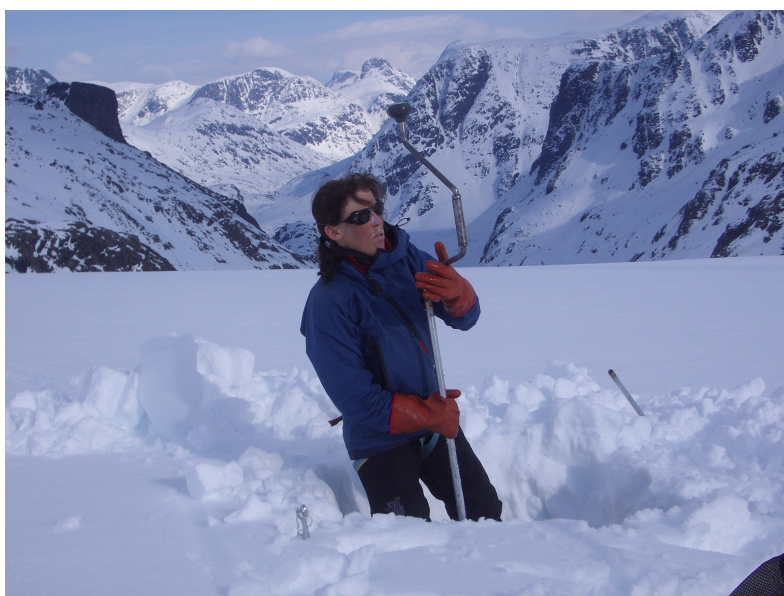
Figure 12-1 Drilling of substitute stake in April at position 20. Photo: Hallgeir Elvehøy.
