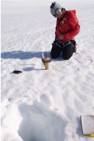
Figure 3-6 GNSS positioning of stakes on 25 th September 2019. Photo: Hallgeir Elvehøy.
