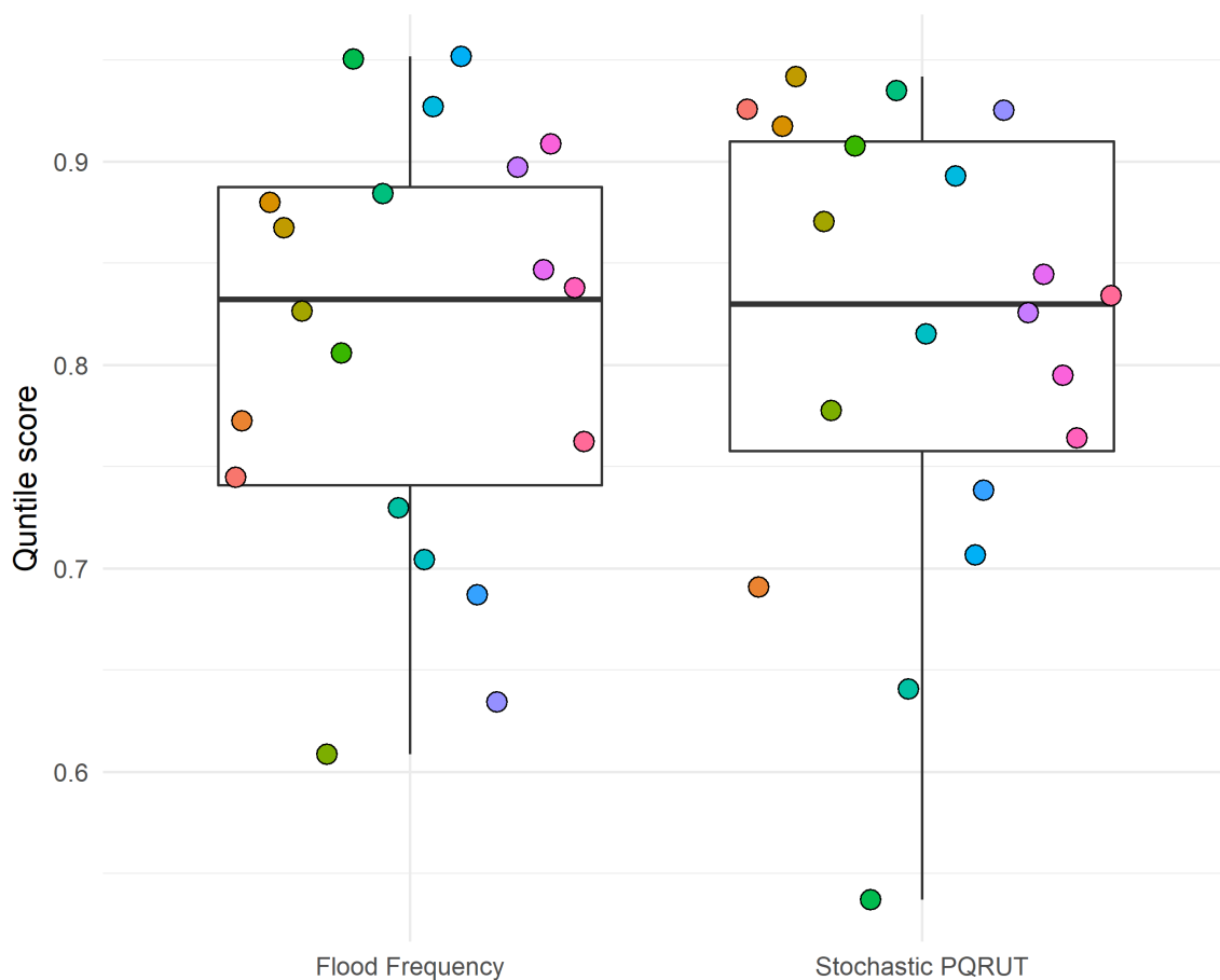
Figure 8. Boxplots of Quantile score, calculated for the Flood frequency analysis and Stochastic PQRUT model, catchments are represented by different colours
