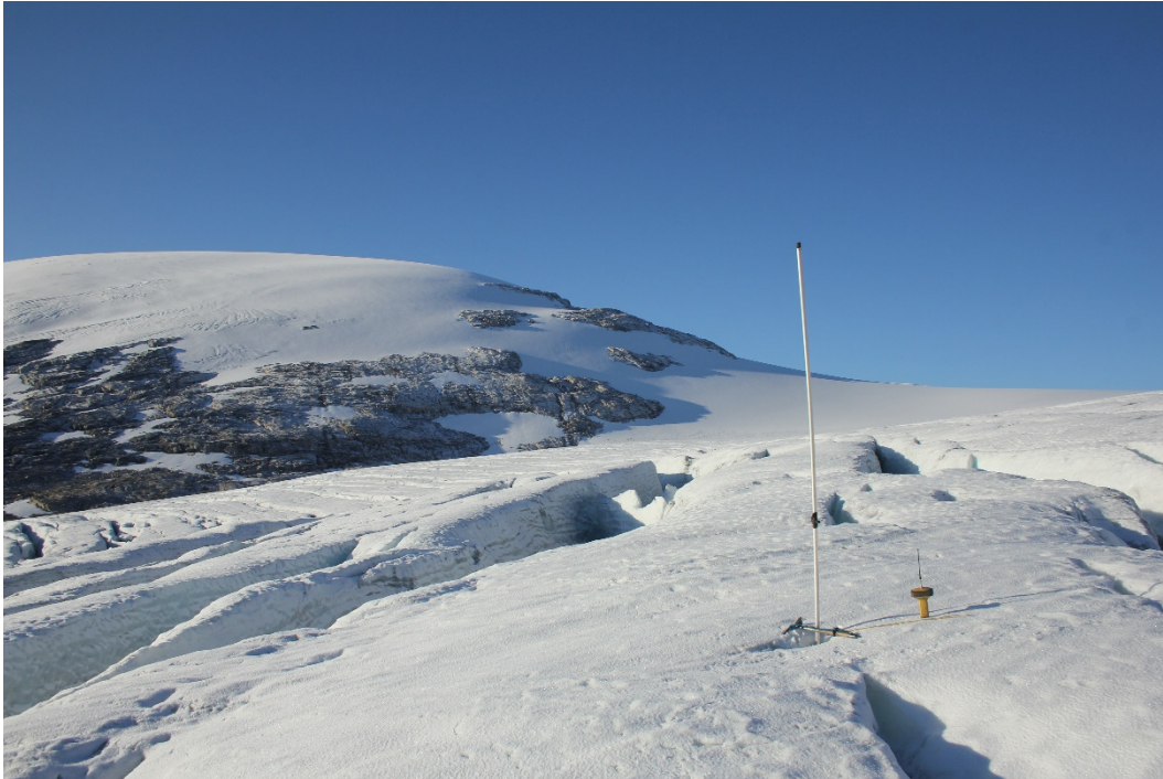
Figure 4-1 Stake A10 on 13 th October 2020. The stake position was surveyed using a GNSS-receiver for glacier velocity calculations. Photo: Hallgeir Elvehøy.
