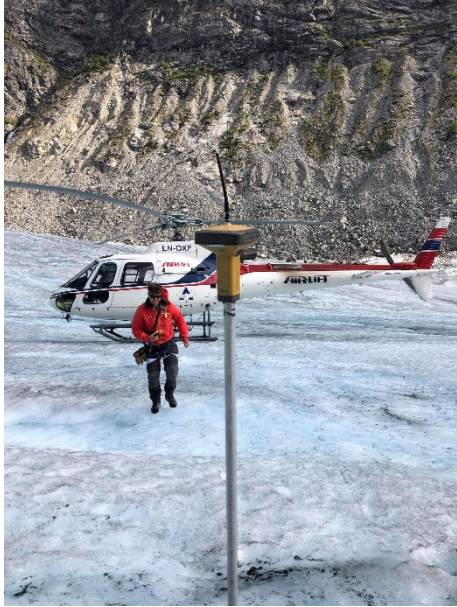
Figure 3-7 GNSS positioning of stakes on 20 th August 2020. Photo: Even Loe.
