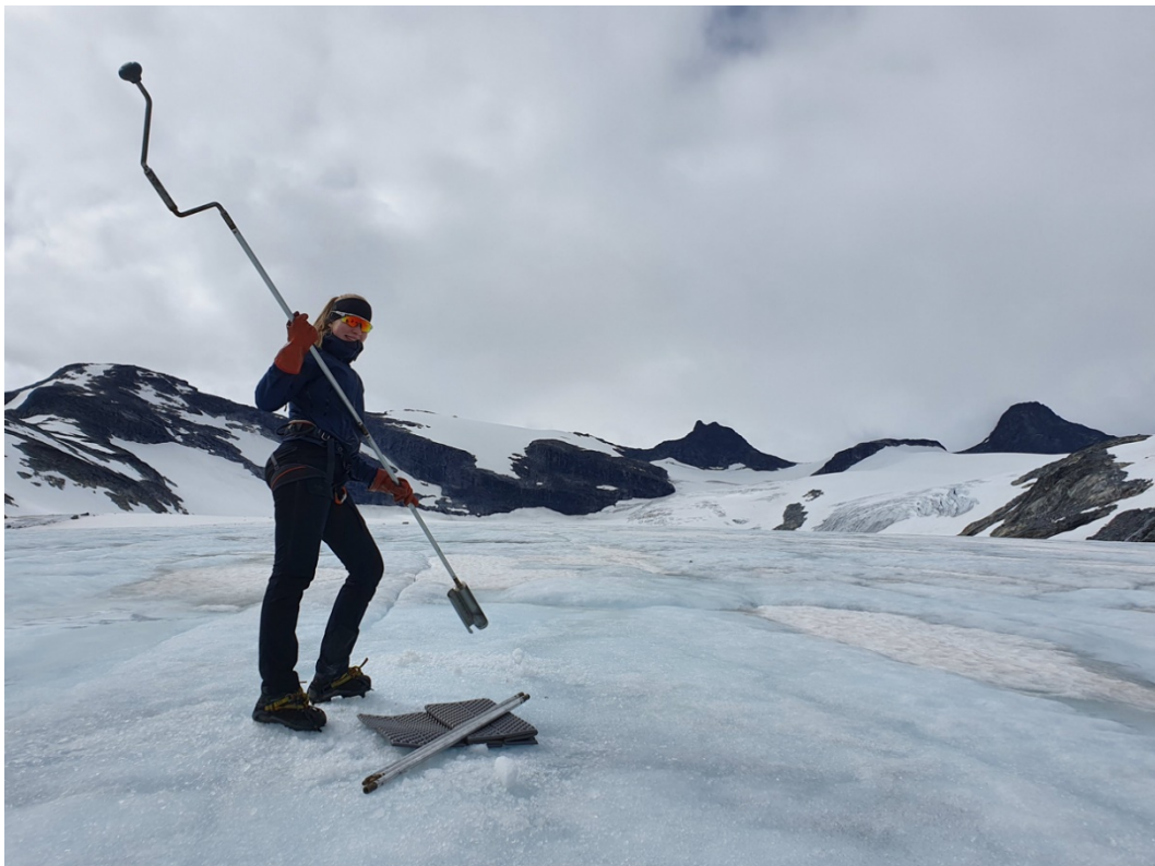
Figure 6-5 Storbreen was also visited on 29 th of July to maintain the stake network. Only stake 1 needed redrilling due to much remaining snow at that time. Photo: Liss M. Andreassen.
