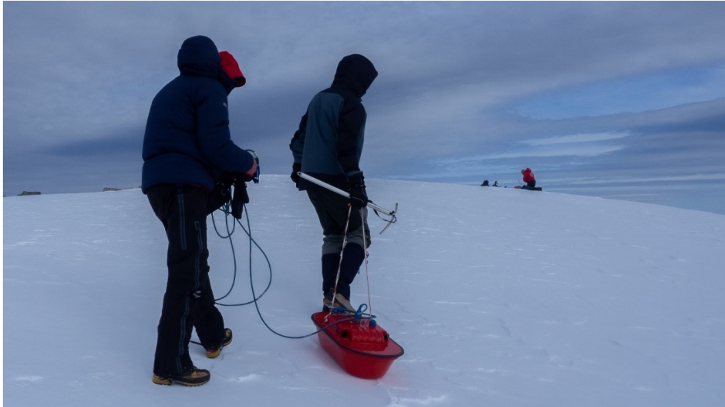
Figure 13-3 Radar survey setup. The red box is the GPR antenna, the control unit is carried by the rearmost operator. In background ice drilling at site A. Photo: Even Lusæter/NRK innlandet.
