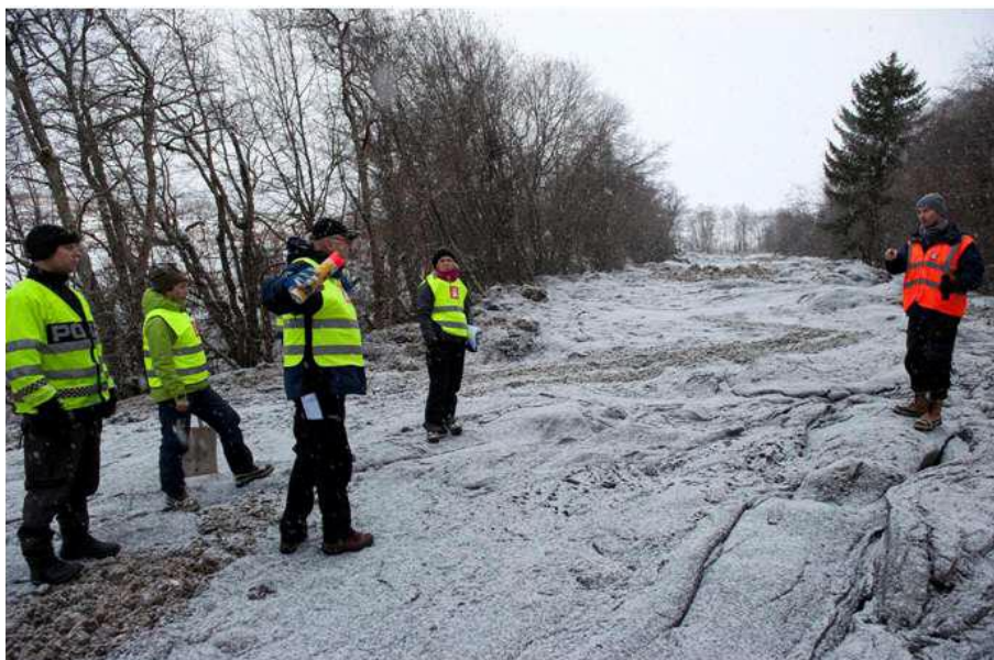
Figure 9. Deposit of the Byneset quick-clay slide completely filling the channel of Brenselbekk. The deposits also dammed tributary brooks. From (Lyche, 2012).
