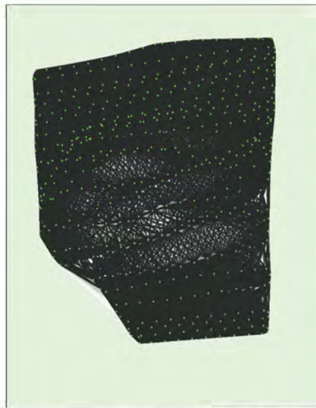
Figure 5: Top view of the image computed positions with a link between matching images. The darkness of the links indicates the number of matched 2D keypoints between the images. Bright links indicate weak links and require manual tie points or more images.
