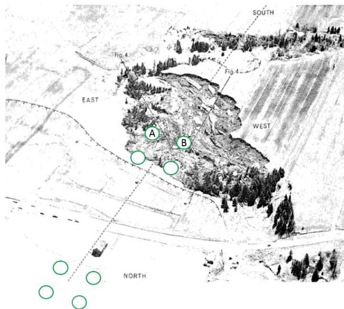
Figur 2-7: The Rigaud landslide area. The route of the proposed north-south power transmission line and the backscarps of two old landslides are superimposed on the print. The green circles indicate the corners of the pylon sites. The landslide occurred while driving the pile for pylon B (after Carson 1979).
