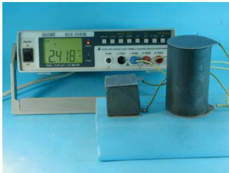
Figure 3.27 Resistivity measurements in the laboratory. Simple lay-out for measurements of electric resistivity and electric anisotropy in a sample.
