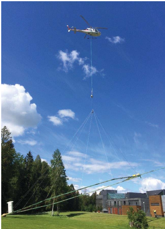
Figure 2.11: AEM equipment (SkyTEM304), take-off at Vestfold University campus.
