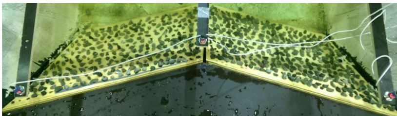
Figur 2.14: Chevron dam, 1:1,5, fra Mortensen (2016)
