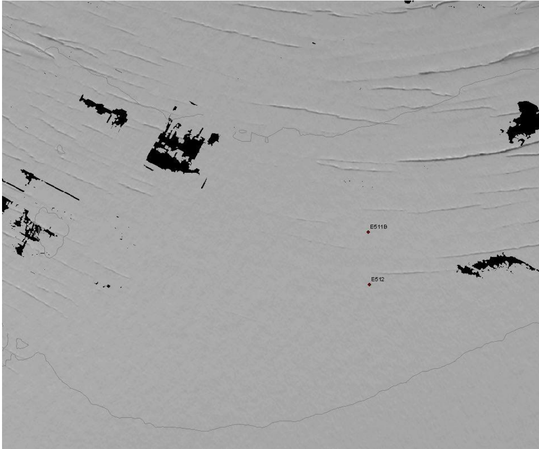
Figure 11-2 Example of missing data in the orthophoto created from the Pleiades images. The width of the plot is 500 m, and the area is located around stake E5 at about 1225 m a.s.l. The vertical distance between contour lines is 10 metres.
