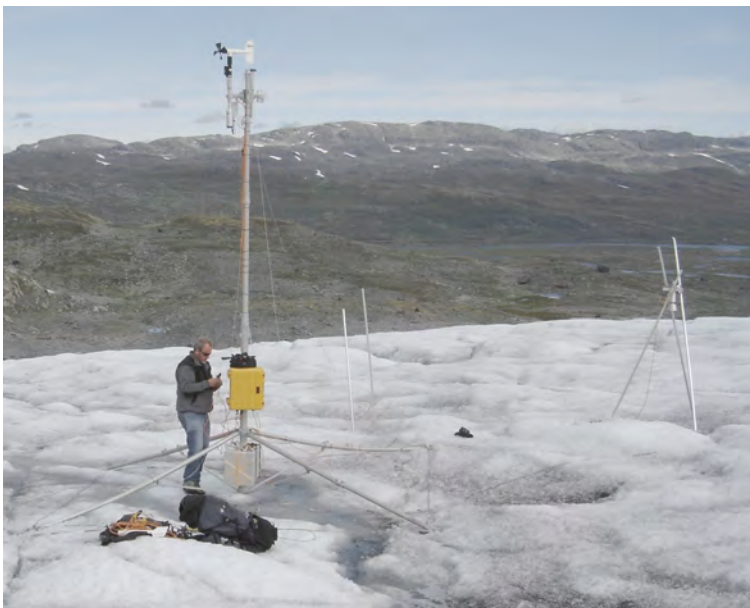
Figure 6-5 The AWS site on Midtdalsbreen on 29 th August 2008. The sonic ranger measuring the changing distance to the ice surface is to the right. Photo: Rianne H. Giesen.
