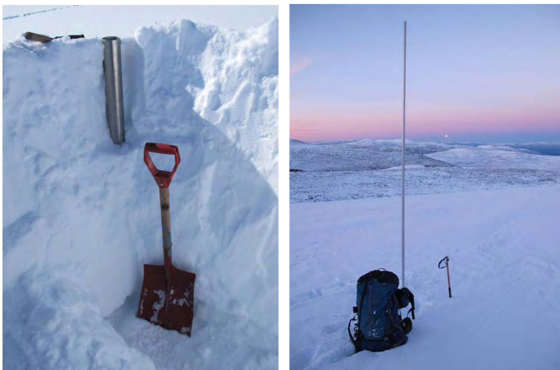
Figure 10-2 Left: Density measurement in snowpit on 4 th May 2010. The snow depth was 1.3 m. Right: Stake 2 at Gråsубreen on 27 th September 2010. Nearly 50 cm of fresh snow covered the surface. Photos: Liss M. Andreassen.
