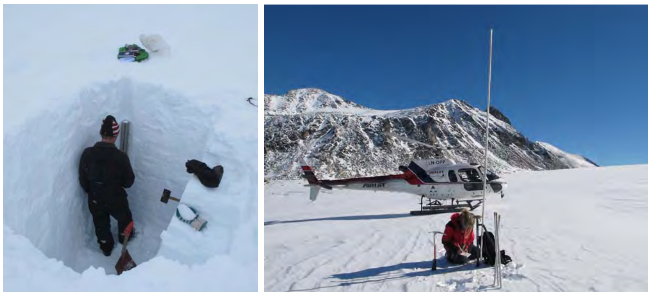
Figure 9-2 Field work 2010. Left: density measurement in a snow pit on 7 th May. Right: Ablation and position measurement on 28 th September. Photos: Liss M. Andreassen and Solveig H. Winsvold.
