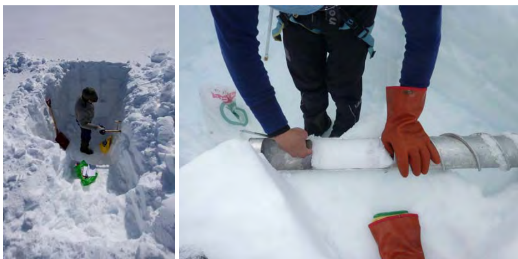
Figure 1-1 Snow density is usually measured by using a sampling cylinder in a snow pit down to 1.5 m depth (to the left) and completed with a coring auger down to required depth, preferably S.S. (to the right). Photo: Ragnar Ekker (left) and Hallgeir Elvehøy (right).
