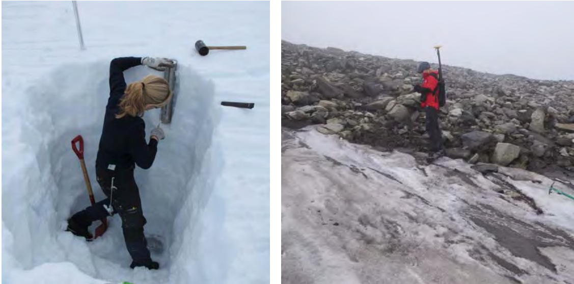
Figure 8-3 Field work: density pit at Juvfonne on 19 th May 2010 (left) and mapping the extent using GNSS measurements on the ice patch on 25 th August 2010 (right). Photos: Atle Nesje and Trine Fjeldstad.
