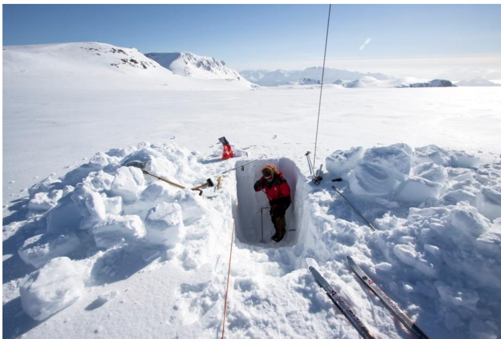
Figure 1-1 Snow density measurements on Langfjordjøkelen in May 2011. Photo: Ragnar Ekker.
