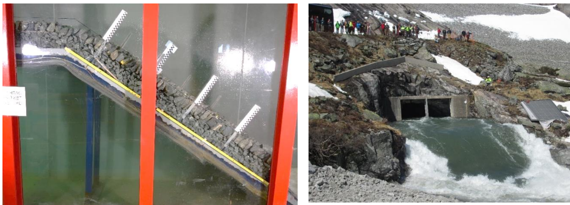
Figure 3. (Left) Sideview of the model setup in the laboratory with placed riprap (Photo: NTNU). (Right) Test with full-scale riprap stones in 2015 (in the Stavanger ICOLD Congress Technical tour).
