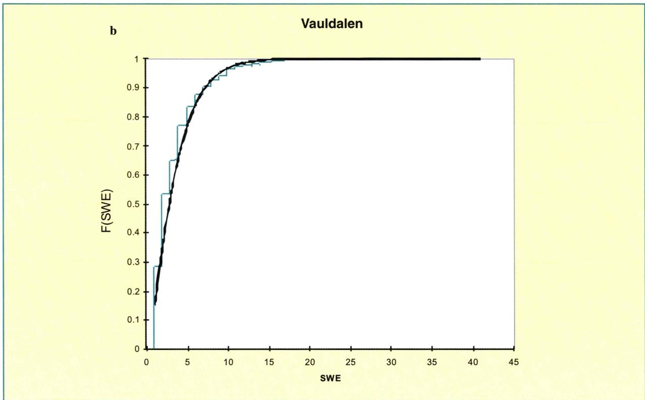
Figure 5. Gamma distribution is fitted (thick solid line) to observed daily values for precipitation station 1040 (a) and snow pillow Vauldalen (b). Parameters for the gamma distribution are found in Table 1 (Vauldalen) and Table 2 (1040).
