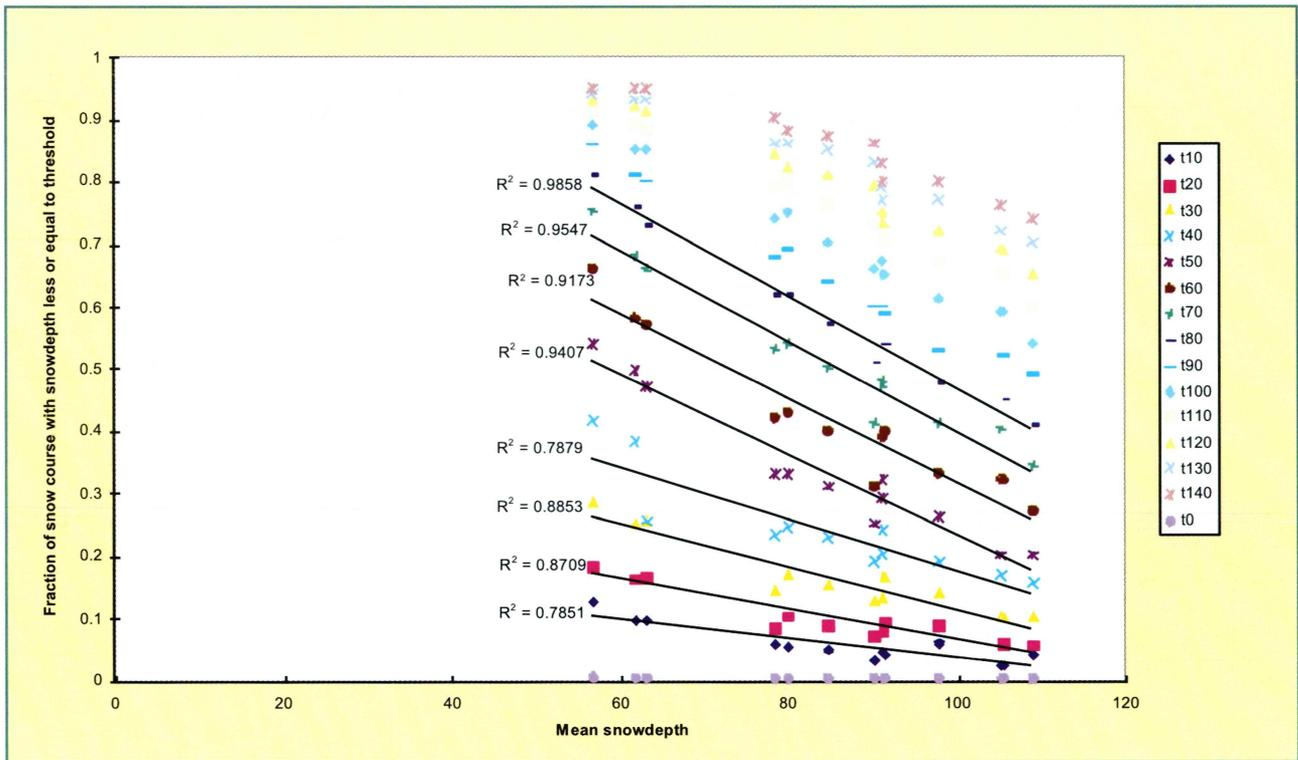
Figure 1. Linear regression lines fitted to fractional areas less or equal to threshold of snowcourses. We note that threshold zero ( $t_0$ ) is uninformative in explaining the mean snowdepth.
