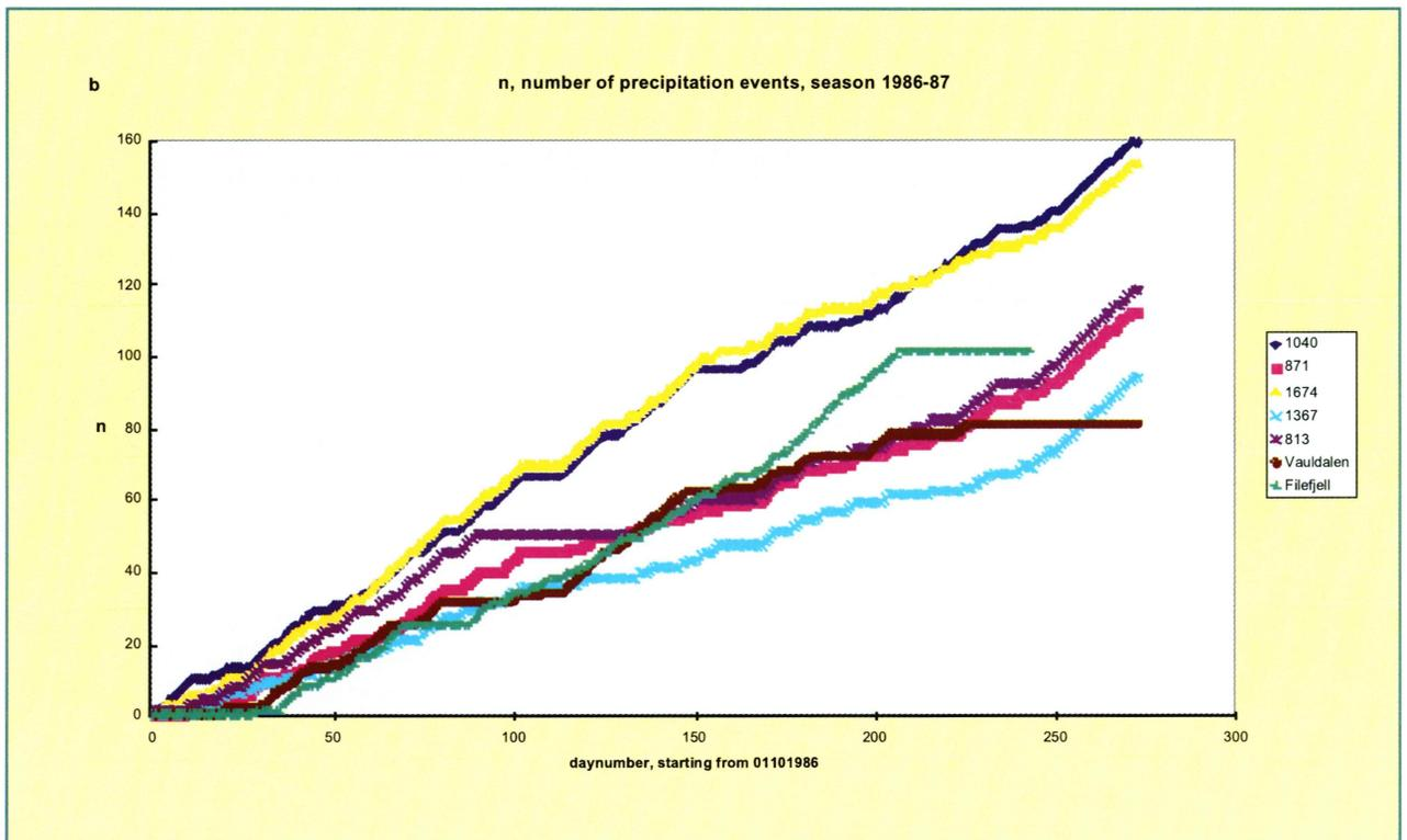
Figure 7. Showing the number of precipitation events registered at precipitation stations, 1040, 871, 1674, 1367, 813 and at the snowpillows Vauldalen and Filefjell. a) Winter 1984-85, b) Winter 1986-87.
